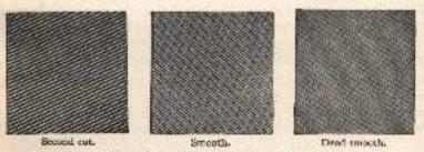
Fig. 83.-Five main graduations of double-out files (12 inch size),
