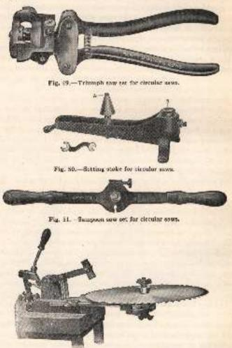
Fig. SI,-Machine for setting circular assoc
