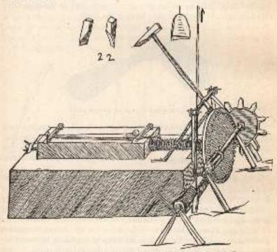
Fig. 96. Leanardo de Vinci's invention for cutting files, 1505 A. D.
