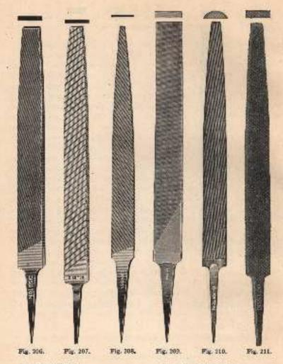
Fig. 206, — Mill File. Fig. 207, — Perfection Shear Tooth File. Fig. 208, — Warding File. Fig. 109 — Lathe on File. Fig. 210. — Half round File for solder. Fig. 211. — Fist Aluminum File.
