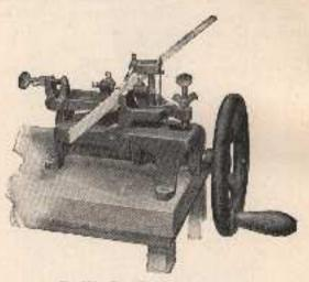
Fig. 177. Band Saw Setting Mochine.
