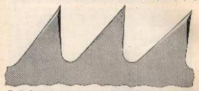
Fig. 40. Bowd and angle of teeth of circular cross cut saw for softwood, magnified.
