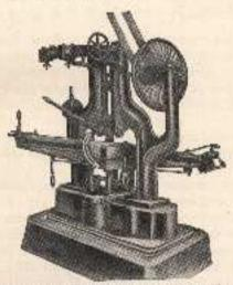
Fig. 97.-First genetical file-cutting machine. Invented by E. Bernst,
