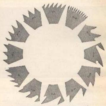
Fig. 73.-Scandard acctions of Distron circular any teeth.
