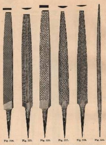
Pig. 234.—Flat Wood File. Pig. 225.—Calmet File. Pig. 235.—Flat Wood Rosp. Fig. 227. Holf-round Word Rass. Fig. 227. Holf round Cohinet Rasp. Fig. 229. Round Word Rasp.
