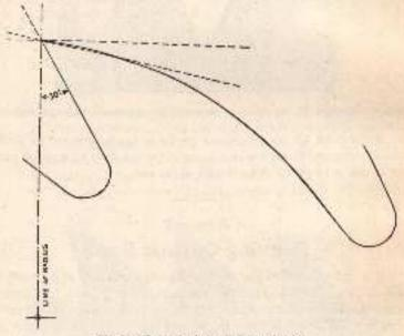
Fig. 44 .- Correctly designed rip any tooth.
