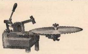
Fig. 188.-Setting machine for circular same.
