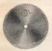
Fig. 54.--Mitre tooth circular saw.
