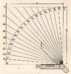
Fig. 111.-Method of setting angles of T bevel.
