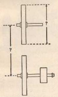
Fig. 136. - Necessary measurements for figuring length of band saw.
