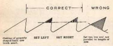
Fig. 33.-Proper setting of narrow band new teeth.
