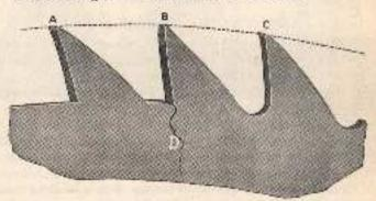
Fig. 42 .--- Crack resulting from square gullet, magnifed,
