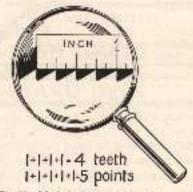
Fig. 27. Method of determining prime per inch.
