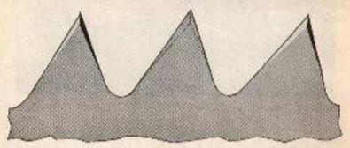
Fig. 41.--Henri and angle of teeth of circular cross cut now for landwood, magnified.
