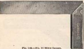
plated profiled to give balance to the tool when the stock projects over the odge of the work, and securely locked square by three strong rivets. For a metal tool this mitre source is commandively light in weight. This tool is square both inside and out. Although available in sizes from 2 to 12 inches, usual school sizes are 6, 8, and 12 inches.
