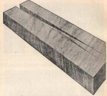
Fig. 13.-Showing progressive action of cross-cut teeth
