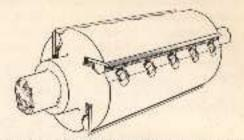
Fig. 104 .- Round cylinder hend with four thin high-speed knives.
