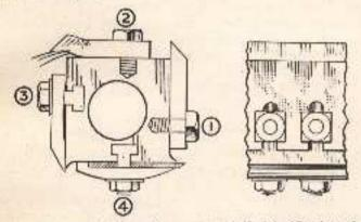
Fig. 102.--1, First method of attaching square head knife; 2, buckling due to flat face; 3, property attached and; with concret bearing surface; 4, adapting head to this highspeed knife.
