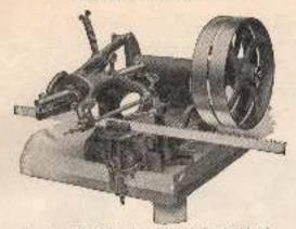
Fig. 175. Band Sow Primg Machine (power driven).
