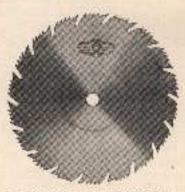
Fig. 181. Combination Circular Saw.
