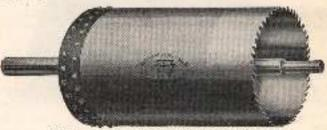
Fig. 71. Cylinder sow for sutting tight barrel staves.
