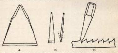
Fig. 94.—A. Chied for handcutting large, wough files; B. chied for centing small, fine files; C. setion of clissel in upsetting teeth.
