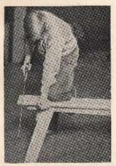
Fig. 15.-Front view of correct cross-cutting position. Note straight line of action.
