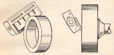
Pig. 106.—Grinding concave bevel on machine imige.
